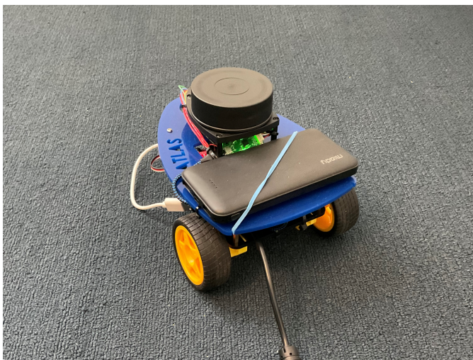
Fig. 1. A close-up view of the robot used. The robot has two motorized wheels and a ball roller. The LiDAR is mounted on top of the robot.
