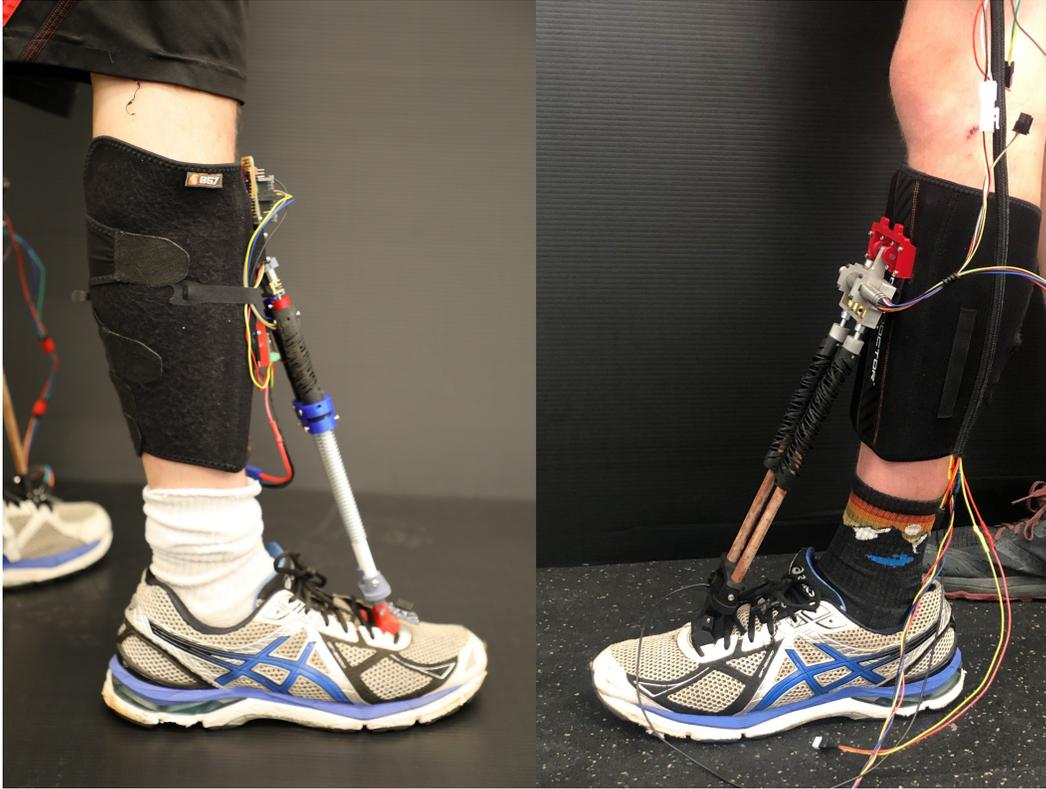
Figure 3.3: **Ankle Exoskeleton Design Comparison.** The drone motor design (left) and the worm gearbox design (right). Both designs share the majority of mounting hardware, but differ in their motor configuration. The worm gearbox design drives both HSAs with a single motor and has electronics located at the hip, while the drone motor design directly drives both HSAs with shin-mounted electronics.
